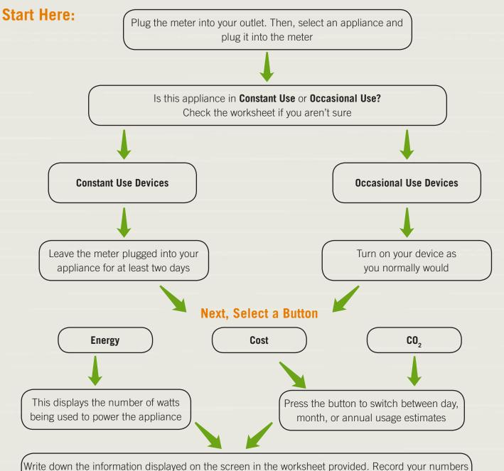
before unplugging the meter, as results will be lost after disconnecting.
